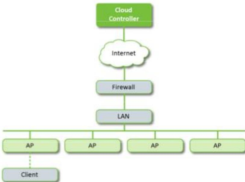
The cloud controller is password protected, and can be accessed through any browser. The controller can:
