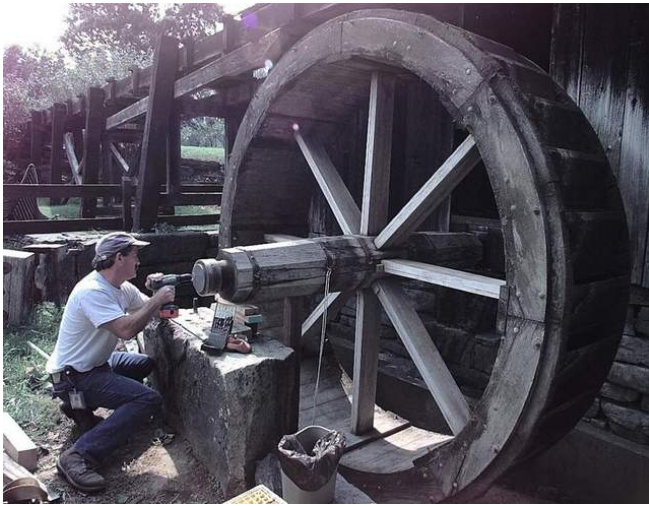
-Loren Cox a lead carpenter at Shelburne Museum, fixes a bearing in a 1991 reconstructed waterwheel at the Museum Monday. The Middle-ages era water wheel is part of an up and down sawmill exhibit. The wheel is constructed with white oak and red cedar which holds up well under wet conditions. shot Monday, September 20, 1999
